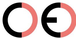
False CE Mark (too far)
